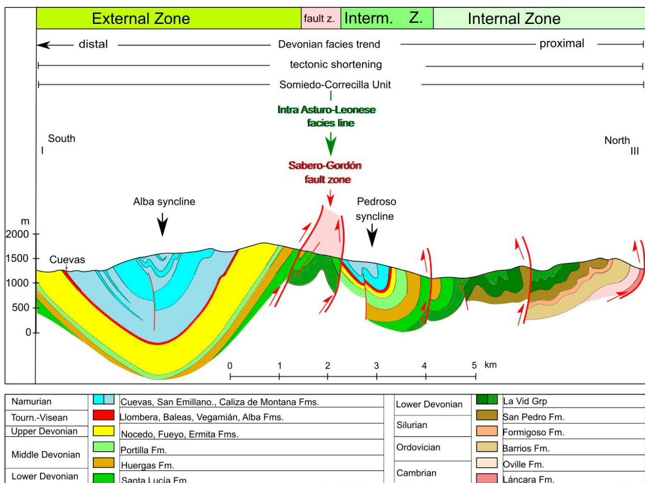
**Figure 10.** Structural N-S cross section of the Bernesga area with Devonian facies trends, tectonic shortening by thrusts, fold and fault zones indicated. Modified after Van Staalduin (1973).
