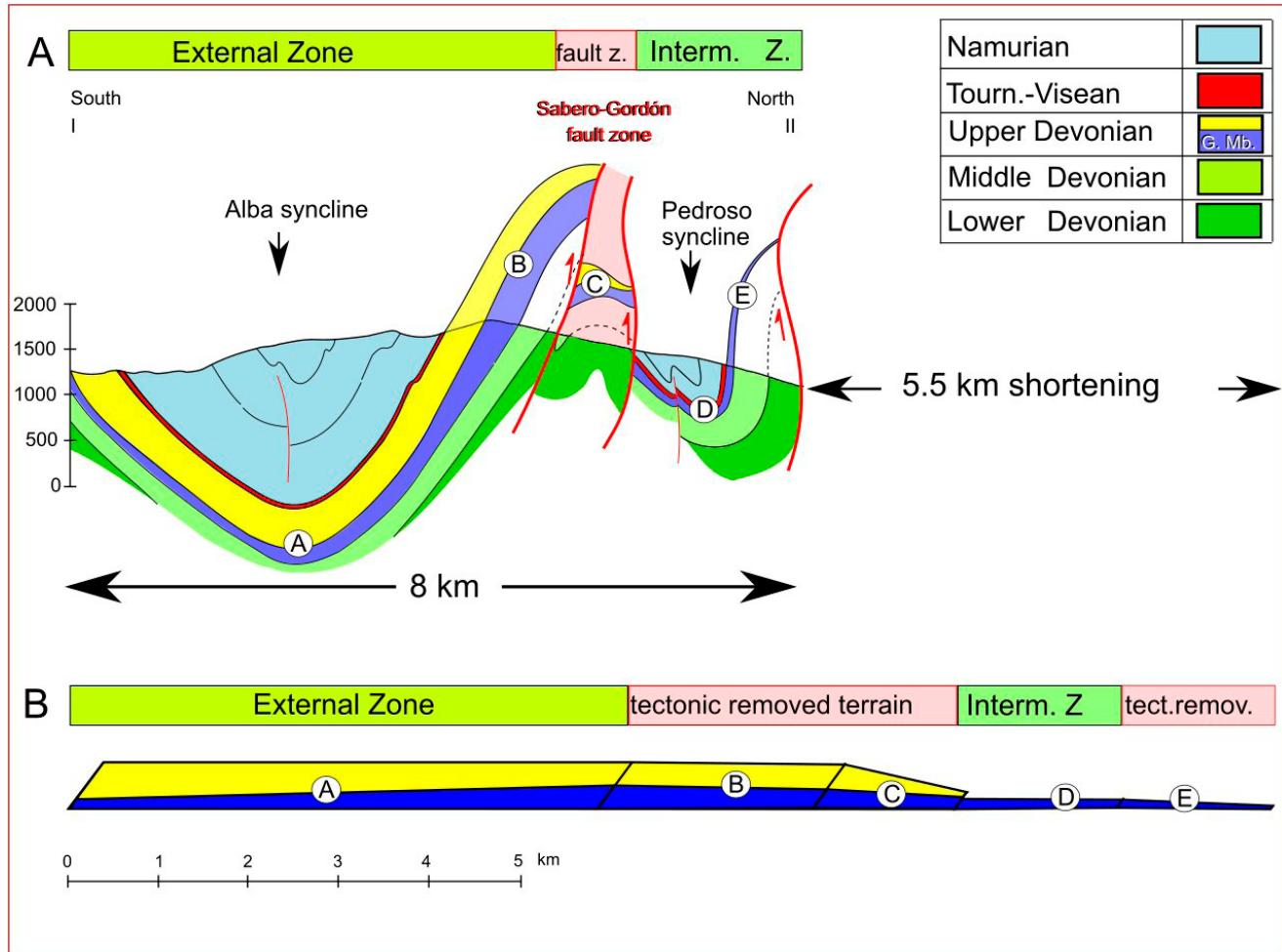
**Figure 11.** Palinspastic reconstruction of the southern part of the Somiedo–Correcilla unit. A) balanced cross section based on Van Staalanduin (1973) (G. Mb.= Gordón Member). B) Upper Devonian restored primary extension.
