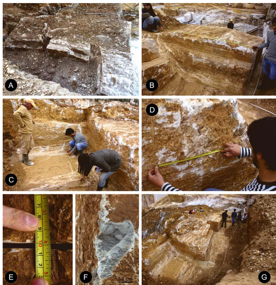
Figure 10. (A) to (G) various stages of cleaning work and data recording in the historic quarry of Fonte da Moura, Pardais, Vila Viçosa. In (F) the recent fracture shows that this is a bluish-grey, veined marble with a white background, commercially known as “Pele de Tigre” (Tiger Skin).
