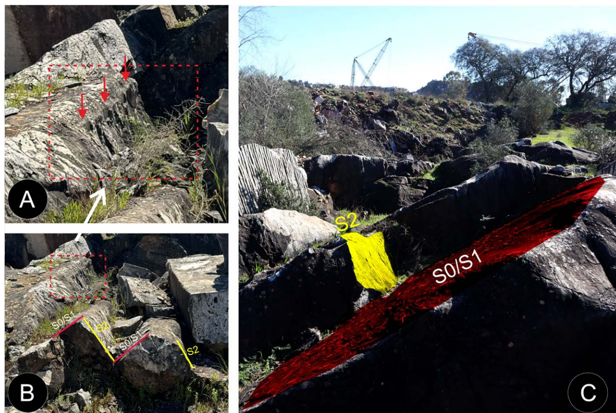
Figure 8. Artificial steps obtained during the marble exploitation. (A) The three red arrows point to the trapezoidal-shaped holes for inserting wooden wedges dug into the plane of the metamorphic foliation. The white arrow points to a cut in a plane that is also parallel to the metamorphic foliation. This cut is the result of multiple subparallel perforations using a pneumatic air hammer, which was quite common before the diamond wire saw was introduced in the 1980s. (B) The combination of these two planes defines a stepped section that is clearly visible throughout the quarry. (C) The banding plane ( S_0/S_1 ) defines gentle dipping planes to the north, while the regional metamorphic foliation ( S_2 ) dips strongly to the south.
